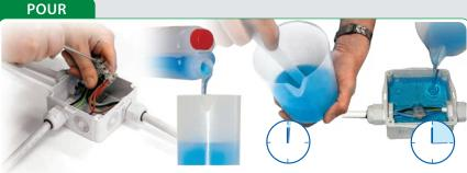
You can use the Magic Power gel supplied in the two-component bottle in a 1:1 ratio by simply pouring it after mixing into the box supplied in the kit, to protect and seal internal connections. The gel cross links in just 15 minutes, but the box can be energised immediately.
